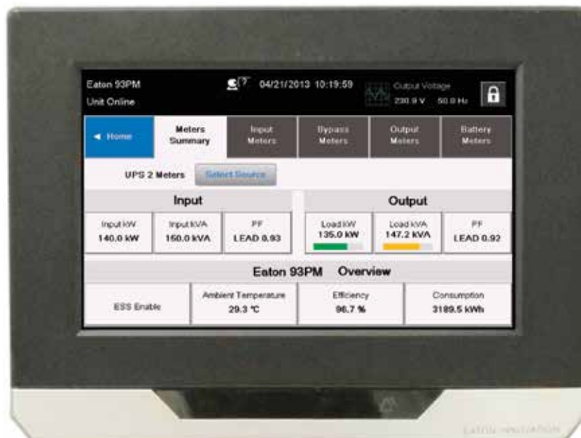
93PM 7' Touch Screen Colour LCD Interface
